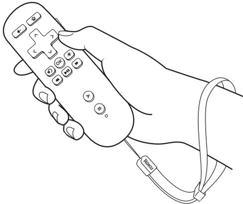
**Buckle up:** Open the lever on the strap lock and place your hand through the wrist strap. Hold the remote firmly in your hand. Slide the strap lock up so that the strap will not fall off your wrist. Do not over-tighten the strap lock so that it's uncomfortable. It should just be tight enough to hold the wrist strap in place. Close the lever to hold the strap lock in place.
